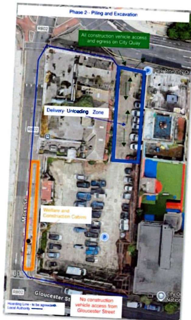
Site cabins move to Moss Street to facilitate piling and excavation works
